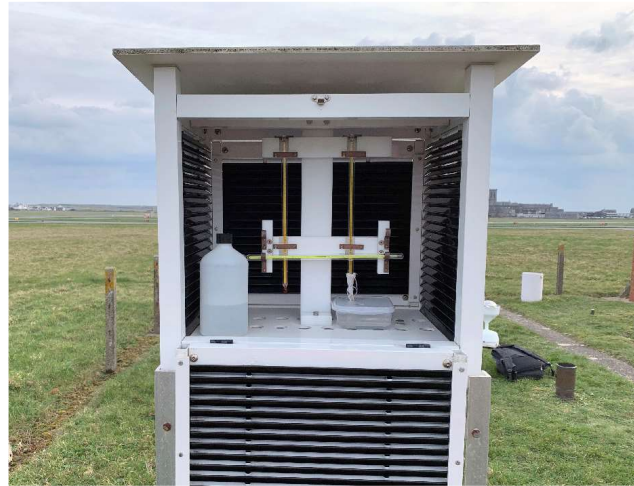
Stevenson screen showing thermometers
