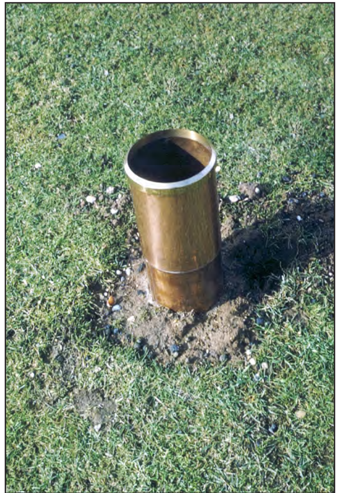
Left: Example of a rainfall card. Right: Standard rain gauge (used for collecting and measuring rainfall).
